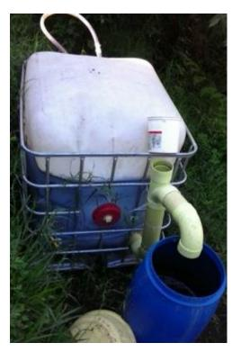
water to leach the materials will gradually result in a build up of salts and other inhibitory compounds in the liquid which will eventually kill the bacteria needed for the reaction. We therefor advise that at least every 5<sup>th</sup> time you remove the effluent from the reactor, you remove it from the system (use this water for fertilizer!) and fill the new leaching container with fresh water.
