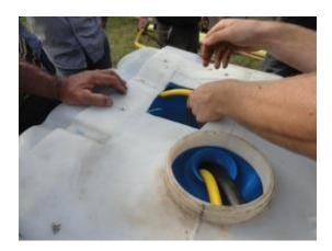
The lid with the two containers attached and the connected hoses are then placed into the open 1000 liter container, with the lid facing downwards.
